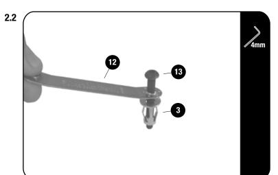
Insert a M6 x 30 Button Head Bolt (Item 13) into the Jack Nut Tool (Item 12) and loosely fit a Jack Nut (Item 3) to the button head bolt as shown.
