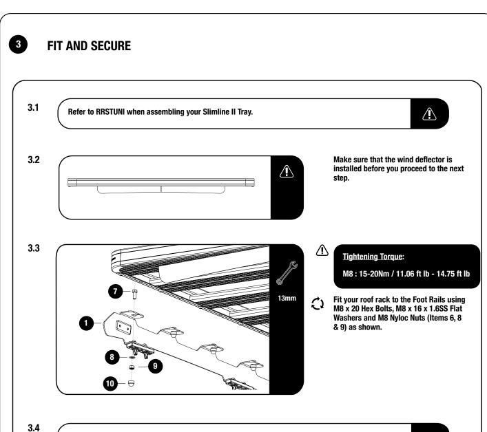
Center the rack and tighten fully. Use M8 Nut Caps (Items 10) to finish off the nuts.
