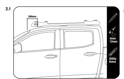
Starting at the top edge of the vehicle's windscreen, measure and mark the dimension as shown onto both LH / RH ditch centre's.
