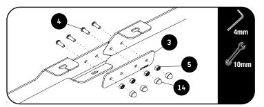
Join the two halves of the Foot Rails
