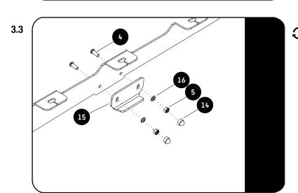
Loosely fit the Support Bracket (Item 15) to the foot rail using M6 x 16 Button Head Bolts, M6 Flat Washer and M6 Nyloc Nuts (Items 4, 5 & 16).
