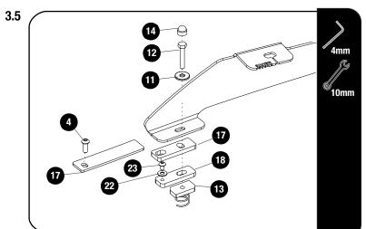
Apply a bead of silicone on each Hex Bolt inserting it into the roof.
