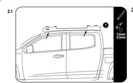
With the Factory ditch trim removed (Keep aside for later use). Place the foot Rail (Item 1) on to the ditch, aligning the rear hole with the factory hole in the ditch.Mark the 1st and 4th hole in the Foot Rail on the ditch.
