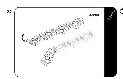
Apply a bead of silicone on the 4 Nut Plates (Item 10) before placing and securing the nut plates. This will bond the Nut Plates in place, so that the headliner does not need to be removed in future, should you want to remove the rack.
