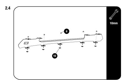
Once all the bolts are fitted to the nut plates (Item 10) Fully tighten all the bolts and place the M6 nut Caps (Item 8) on all the bolts
