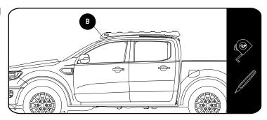
Place the foot rail on the vehicle's roof lining up the front slot center with the mark you made earlier and mark the centre of the remaining three slots.
