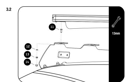
Secure your roof rack to the Foot Rails using M8 x 20 Hex Bolts, M8 x 16 x 1.6SS Flat Washers and M8 Nyloc Nuts (Items 11, 12 & 13).
