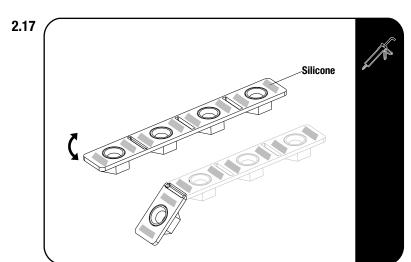
Apply a bead of silicone on the four Nut Plates (Item 6). This will bond the Nut Plates in place, so that the headliner does not need to be removed in future, should you want to remove the rack.
