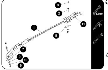
Apply a bead of sealant on the threads of the M8 x 40 Hex Bolts and secure the Foot Rail (Item 1) together with the Support Bracket (Item 11) and the Front and Rear Spacers to the Roof using M8 x 40 Hex Head Bolts, M8 x 19 x 2 Flat Washers and M8 Nyloc Nuts (Items 2, 6 & 10).
