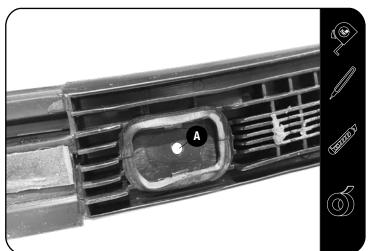
Remove the Ditch Mold from the vehicles roof. Remove the Stud insert from the plastic trim and place the Bottom Spacer (Item 9) into the opening and mark the center of the hole (A).
