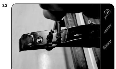
Remove the OEM Rails with Ditch Trim from the vehicles roof by unbolting the nut on the inside of the roof.
