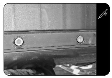
Place a bead of silicone around each of the Jack Nut openings inserted earlier in 2.4
