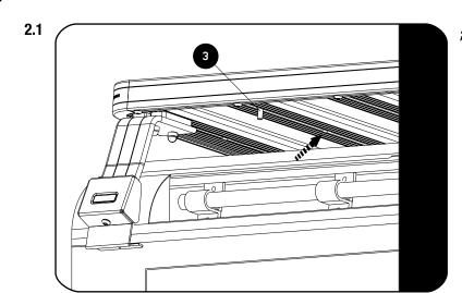
Slide M8 x 20 Hex Bolts (Item 3) into the machined slots on the 2nd, 4th, 6th & 9th slats from the rear.
