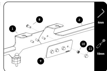
Assemble the front and rear Foot Rails (Items 1 and 2) with the Joiner Plate (Item 9) using M6 x 16 Button Head Bolts and M6 Nyloc Nuts (Items 8, 9, & 11) as shown.
