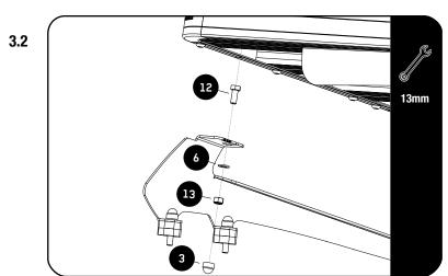
Fit your Roof Rack to the Foot Rails using M8 x 20 Hex Bolts, M8 x 16 x 1.6 Flat Washers and M8 Nyloc Nuts (Items 6, 12 & 13).
