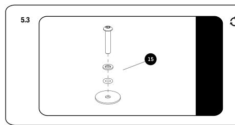
Should you wish to remove your rack, you will need to plug the holes you drilled in the roof (Step 3.4), using the supplied Sealing Plug Assemblies.
