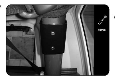
Locate the two threaded holes on the underside of the roll bar and fasten the two halves of the Roll Bar Clamps (Items 3 & 4) to the roll bar using M6 x 19 x 1SS Flat Washers and M6 x 20 Hex Bolts (Items 7 & 10). Place the Outer Roll Bar Clamp (Item 3) first, followed by the Inner Roll Bar Clamp (Item 4).
