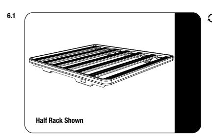
With the help of a friend, flip the Tray end over end so that it is in the upright position. (The Tray is flipped end over end so that bolts and brackets do not slide left and right).
