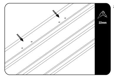
Change the 4mm drill bit to a 22mm hole saw. From the outside of the vehicle, drill all the 4mm holes (8 in total) out to 22mm.
