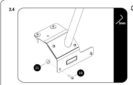
Place two Spacers 19x12x12 (Item 11) into the two side recesses shown in 2.2, between the Front Pillar Assemblies and the Corner Cover.
