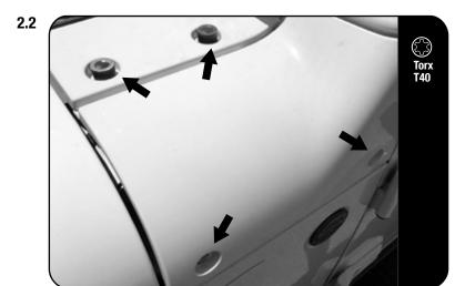
Using a T40 Torx Wrench, remove the four bolts holding the Corner Cover in place.
