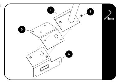
Assemble the LH Pillar Assembly (Item 1) to the Mount Bracket E and D (Item 5 & 6) using M8 x 16 Button Head Bolts (Item 9)
