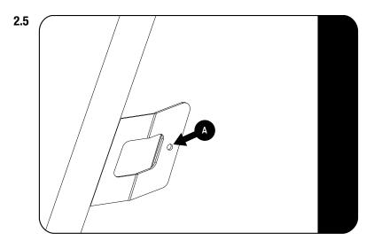
Remove the backing of the double sided tape (A) and press it firmly against the A-pillar.
