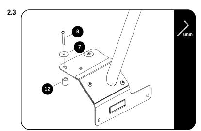
Apply a small bead of thread lock to the button head screws.
