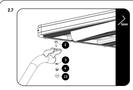
Fit your Roof Rack to the Front Pillar Brackets using M8 x 20 Hex Head Bolts, M8 Flat Washers and M8 Nyloc Nuts (Items 2, 3 & 4) as shown.
