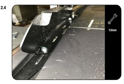
Place the assembled Foot Rails from Step 2.3 over the studs in the vehicle's ditch. Loosely fit the Foot Rails using M8 x 16 x 1.6SS Flat Washers and M8 Nyloc Nuts (Items 9 & 10).
