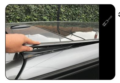
Before starting the fitment you need to remove the front and rear Ditch Covers from the vehicle's roof using a medium flat screw driver.
