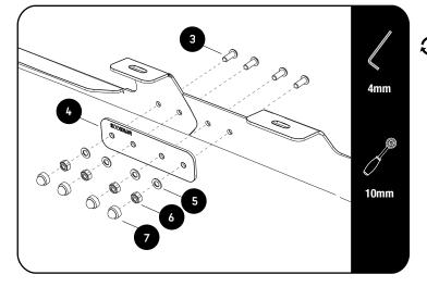
Join the Front LH and Rear LH Foot Rail (Items 1 & 2) with the Joiner Plate (Item 4) using M6 x 16 Buttom Head Bolts, M6 x 12 x 1SS Flat Washers and M6 Nyloc Nuts (Items 3, 5 & 6). Place M6 Nut Caps (Item 7) on all the
