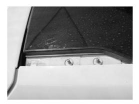
( **B** ) Looking at the front of the vehicle's roof, carefully remove the plastic cover either side to expose the two mounting studs.
