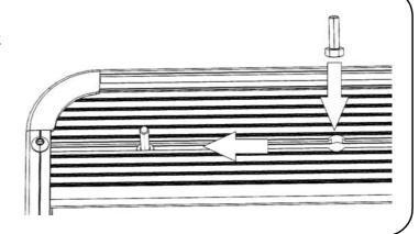
( **B** ) With your rack still upside down from Step 3A, slide a M8 x 20 Hex Bolt (Item 4) into the end of Slats 3, 7 & 8.
