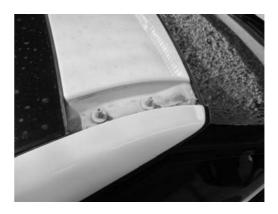
Place the Foot Rails onto the vehicle's roof, lining up the mounting holes in the bottom of the Foot Rails with the studs in the vehicles roof. The Product Sticker must go to the rear of the vehicle and must be facing outwards. Push the Foot Rails as far back as possible and secure them to the vehicle using eight M8 x 19 Flat Washers and eight M8 Nyloc Nuts (Items 2 & 3). Place a M8 Nut Cap (Item 1) over each M8 Nyloc Nut.
