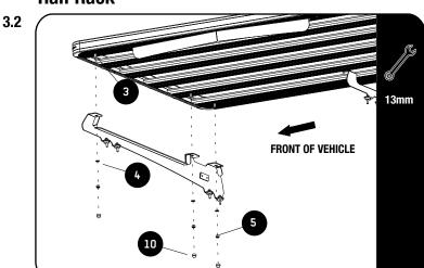
Fit your Roof Rack to the Foot Rails using M8 x 20 Hex Bolts, M8 x 16 x 1.6 Flat Washers and M8 Nyloc Nuts (Items 3, 4 & 5).
