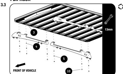
3.4 Center the rack and tighten fully. Use M8 nut caps (Item 10) to finish off the nuts.
