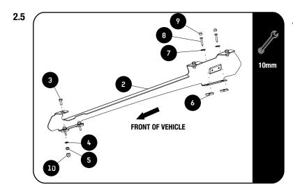
Place silicone around the mounting holes, place the Spacers (Item 6) over the holes, then assemble the Footrail (Item 2) with the M6 x 30 Hex Bolts (Item 8) and M6 x 20 x 2 Flat Washers (Item 7) - placing some silicone on the threads before assembly.
