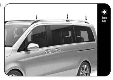
Before you start with the fitment of the Foot Rails (Items 1 & 2), you will need to remove the factory roof rails.
