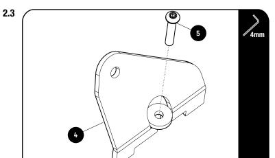
Place the Rear Foot Assembly (Item 4) into the ditch where the Cap screw was removed and bolt the Front Foot Assembly using the M6x35 Button Head (Item 5) Screw as shown.
