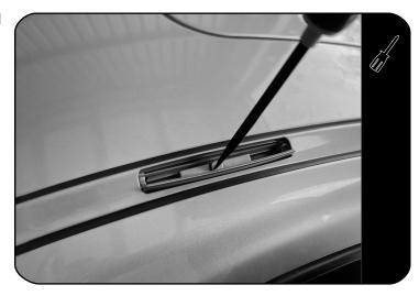
Start by removing the 4 Cap screws using a Flat Screw driver as shown.
