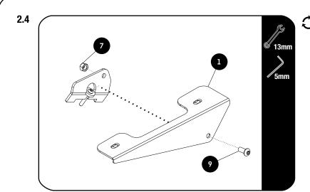
Loosely assemble the Front Top Bracket
