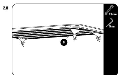
Fully Tighten The M8 x 20 Button head screws fitted in 2.4 & 2.5 and place the M8 Nut cap (Item 8) onto the M8 Nyloc Nut.
