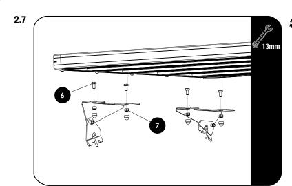
Fit your roof rack to the Foot Rails using M8 x 16 Hex Bolts, and M8 Nyloc Nuts (Items 6 & 7) as shown.
