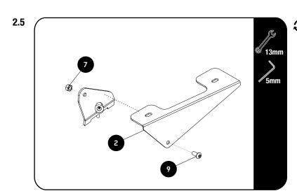
Loosely assemble the Rear Top Bracket (Item 2) to the Front Foot Assembly fitted in 2.3 using the M8 x 20 Button heas screw and M8 Nyloc Nut (Item 9 & 7).
