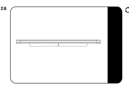
Make sure that the wind deflector is installed before you proceed to the next step
