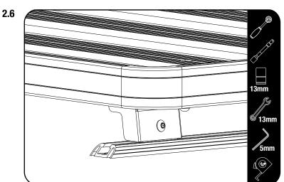
Before tightening the Foot Base to the tracks, position the Rack so that it sits level to the ground, not the vehicle's roof line, or slanting slightly down toward the front.
