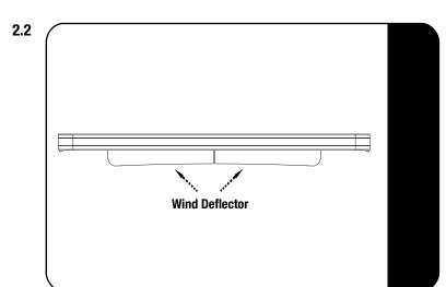
While your Rack is flipped make sure that the wind deflector is installed on the first slat.
