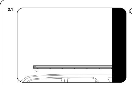
Place your Front Runner Roof Rack over your vehicle and find the best position. The Rack should sit level to the ground, not the vehicles roof line, or slanting slightly down toward the front.
