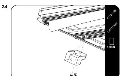
Assemble the Foot Top (Item 1) to the Rack as shown using M8 x 20 Hex Bolts inserted earlier in 2.1 and M8 Nyloc Nuts (Items 4 & 7).
