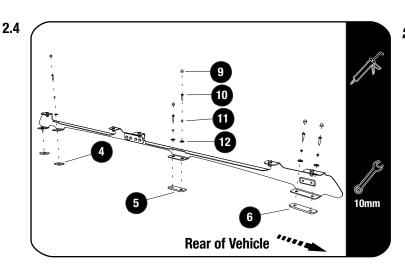
Place the Front, Middle and Rear Spacers (Items 4, 5 & 6) over the factory mounting holes. Apply Silicone to the factory holes before placing the Foot Rail onto the spacers.
