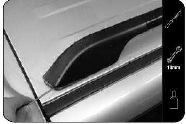
Using a pannel tool, remove the front, middle and rear covers from both roof rails.
