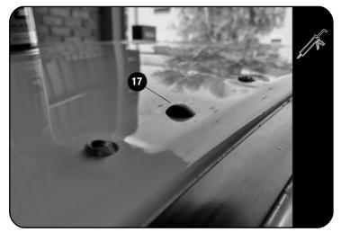
Apply a bead of silicone around the locating holes of the factory rubber pads before inserting 4 Rubber Inserts (Item 17) as
