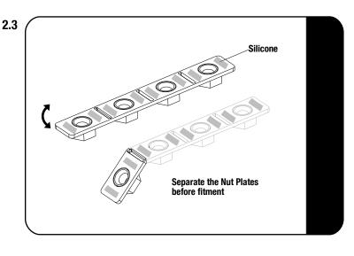
Apply a bead of silicone on the four Nut Plates (Item 10). This will bond the Nut Plates in place, so that the headliner does not need to be removed in future, should you want to remove the rack.
