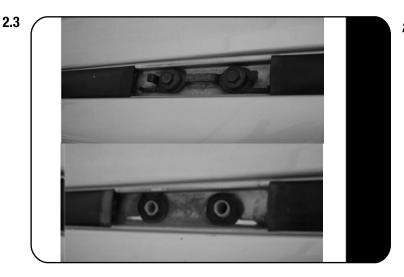
Remove the two bolts and steel bracket below each Plastic Cover ( C ) removed in Step 2.2.
