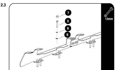
Secure the Foot Rails to the vehicle using the M8 x 40 Hex Bolts, M8 Spring Washer and M8 x 19 Flat Washers (Items 5, 6, 8).
