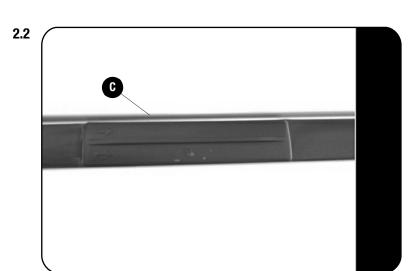
C) Locate and remove the eight Plastic Covers (four each side) in the Ditch Moulding of the vehicle's roof. This is done my pushing the covers in the direction of the arrows found on the covers, and lifting.
