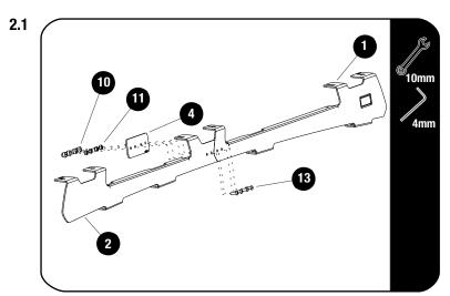
Loosely join the Front and Rear Foot Rails (Items 2 & 1) together using the M6 x 16 Button Head Bolts, M6 Nyloc Nuts and Joiner Plates (Items 13, 11, 4). Tighten all the Nuts and Bolts and place a M6 Nut Cap (Item 10) over each Nyloc Nut.
