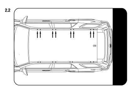
Place the assembled Foot Rails onto the vehicle's roof, lining up the mounting holes in the bottom of the Foot Rails with the mounting points on the vehicle. The Product Sticker must go to the rear of the vehicle and must be facing outwards.
