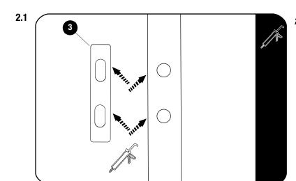
Clean the area around the threaded holes in the vehicle's roof using a rag and some methylated spirits / denatured alcohol. Place some silicone around and into each threaded hole in the vehicle's roof. Do the same around and in the two cut-outs in each of the Spacers (Item 3) as shown. Position the Spacers into the vehicle's gutters, lining up the cut-outs in the Spacers with the threaded holes in the vehicle roof.
