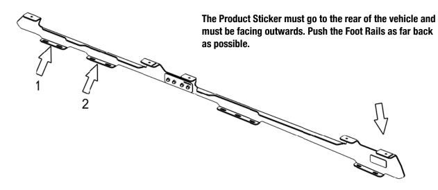
Secure the Foot Rails to the vehicle using the M8 x 40 Hex Bolts, M8 Spring Washer and M8 Flat Washers (Items 2, 3, 4). Place a M8 Nut Cap (Item 1) over each Bolt Head once fastened.
