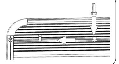
( **B** ) With your rack still upside down from Step 3A, slide a M8 x 20 Hex Bolt (Item 5) into the end of Slats 4, 5, 9, 10.
