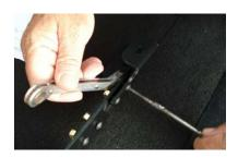
( **B** ) Locate and remove the six Plastic Covers (three each side) in the Ditch Moulding of the vehicle's roof. This is done my pushing the covers towards the front or rear of the vehicle and lifting.
