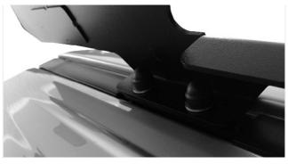
( **F** ) Secure the front Spacers to the vehicle using the remaining M8 x 40 Hex Bolts, M8 Spring Washer and M8 x 19 Flat Washers. Place a M8 Nut Cap (Item 1) over each Bolt Head once fastened.
