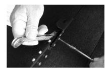
( **B** ) Remove the two end caps, front and rear on each Roof Rail and undo the bolts as indicated by the arrows securing the Roof Rails to the vehicle.
