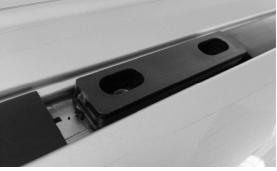
Place the assembled Foot Rails onto the vehicle's roof, lining up the mounting holes in the bottom of the Foot Rails with the mounting points on the vehicle. The Product Sticker must go to the rear of the vehicle and must be facing outwards. Push the Foot Rails as far back as possible.
