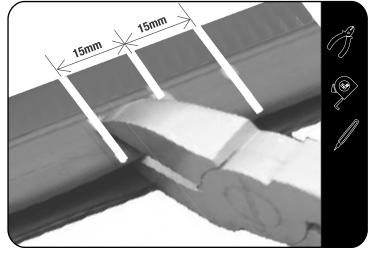
You need to remove sections from the underside of the ditch molding - so you need to transfer the hole centers to the underside of the molding. Mark a line 15mm either side of the center lines marked in step 2.1.
