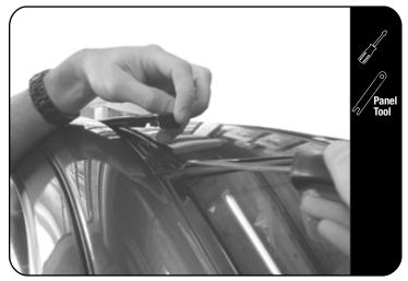
Using a panel tool or flat screw driver start from the front of the vehicle, lift and remove the two ditch moldings running along either side of the roof.
