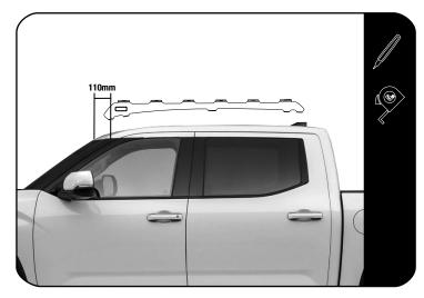
Starting at the top edge of the vehicle's windscreen, measure and mark the dimensions as shown onto each of the ditch trim pieces.
