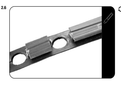
Drill a pilot hole from above using your original marked holes - then open the holes to 22mm using a punch, step drill or hole saw
