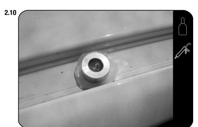
Clear the area around each mounting point in the ditch using a rag and denatured alcohol.
