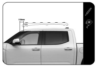
Starting at the top edge of the vehicle's windscreen, measure and mark the dimensions as shown onto each of the ditch centers.
