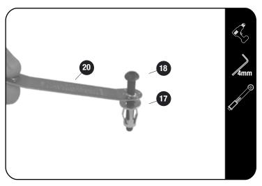
Insert a M6 x 35 Button Head Bolt (Item 13) into the Jack Nut Tool (Item 12) and loosely fit a Jack Nut (Item 10) to the button head bolt as shown.
