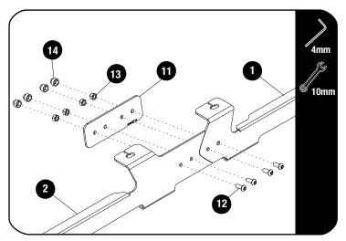
Assemble the Front and Rear Foot Rail (Items 1 & 2) with the Joiner Plate (Item 11) using M6 x 16 Button Head Bolts and M6 Nyloc Nuts (Items 12 & 13) as shown.
