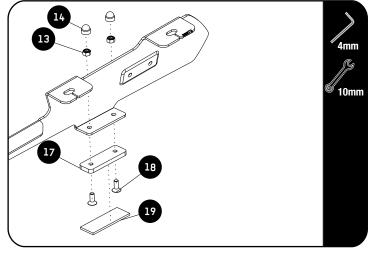
Assemble the Spacer (Item 17) to the Foot Rail using the M6 x 16 counter sunk Bolts together with the M6 Nyloc Nut and M6 Nut Cap (Item 18, 13 & 14) as shown.
