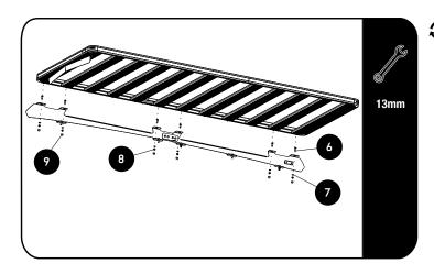
Fit your roof rack to the Foot Rails using M8 x 20 Hex Bolts, M8 x 16 x 1.6SS Flat Washers and M8 Nyloc Nuts (Items 6,7,8 & 9) as shown.
