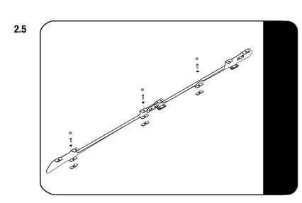
Secure the Foot Rail using the M8 x 30 Hex Bolt, M8 x 19 x 2 Flat washer (Item 15 & 16) together with the 6mm Spacer (item 10).
