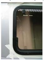
(C) Using a putty knife, cut the sealing tape/silicone holding the window in place. Start at the bottom of the window. Have your friend push against the window from the inside of the vehicle while cutting. Once the tape/silicone has been cut all the way around remove the window.
