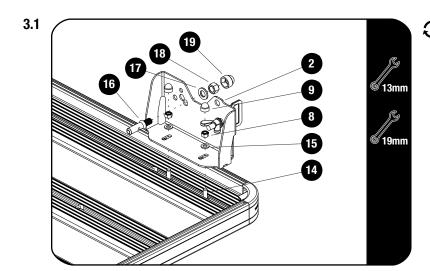
Insert the M12 Pin (Item 16) into the hole in the Base Plate (Item 2) that corresonds with the mounting hole on your hi-lift jack. Fasten with the M12 Flat Washer (Item 17), M12 Nyloc Nut (Item 18) and M12 Plastic Nut Cap (Item 19).
