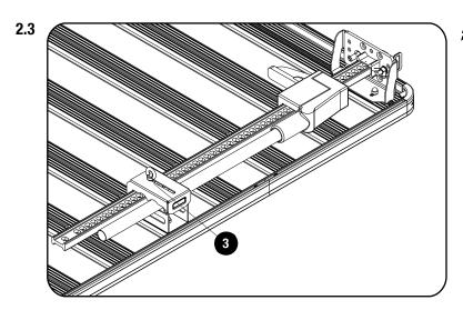
In the orientation seen in Fig 2.3, please note the position of the M8 Threaded Rod (Item 3) and orientation of the Clamp Bracket (Item 1).
