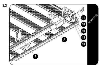
Insert the Hi-Lift Jack (Item A) and fasten it using the Mounting Key (Item 11), the two M10 Flat Washers (Item 10), M8 Spring Washer (Item 12) and the M10 Wing Nut (Item 13). Adjust the brackets so that the M8 Threaded Rod (Item 3) aligns with a hole in the Hi-Lift Jack (Item A). Ensure the Hi Lift Jack (Item A) is square and tighten the M8 Nyloc Nuts (Item 8) and M8 Thin Nut (Item 4), securing the mounting brackets. Place the M8 Nut Caps (Item 9) onto the M8 Nyloc Nuts (Item 8).
