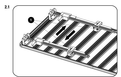
The Hi-Lift Jack can be mounted length-ways anywhere on the rack as seen in Fig 2.1. The Clamp Bracket (Item 1) should always be mounted opening away from you for ease of access.
