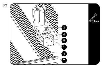
Slide an M8x16mm Hex Head Bolt (Item 7) and a M8 Thin Nut (Item 4) into the slat as shown in Fig 3.2. Loosley mount the Clamp Bracket (Item 1). The M8 Nyloc Nut (Item 8) is fastened to the M8x16mm Hex Head Bolt (Item 7) and the Thin Nut (Item 4) recieves the M8 Threaded Rod (Item 3), followed by another M8 Thin Nut (Item 4).
