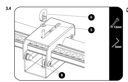
Close the Clamp Bracket (Item 1) and insert a Nylon Washer (Item 5) and M8 Eye Nut (Item 6) onto the M8 Threaded Rod (Item 3). Ensure the Hi-Lift Jack is fitted securely and tighten the button head bolts (Item B) as seen in Fig 3.4.
