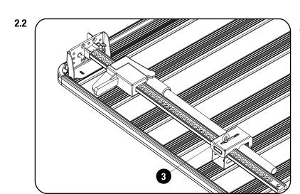
In the orientation seen in Fig 2.2, please note the position of the M8 Threaded Rod (Item 3) and orientation of the Clamp Bracket (Item 1).
