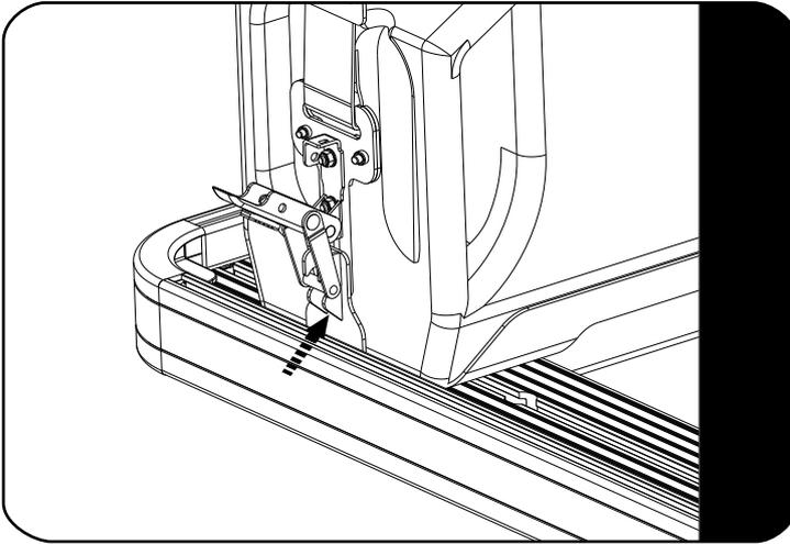
Open the latch and hook it into the catch plate on the Jerry Can Holder Tray.
