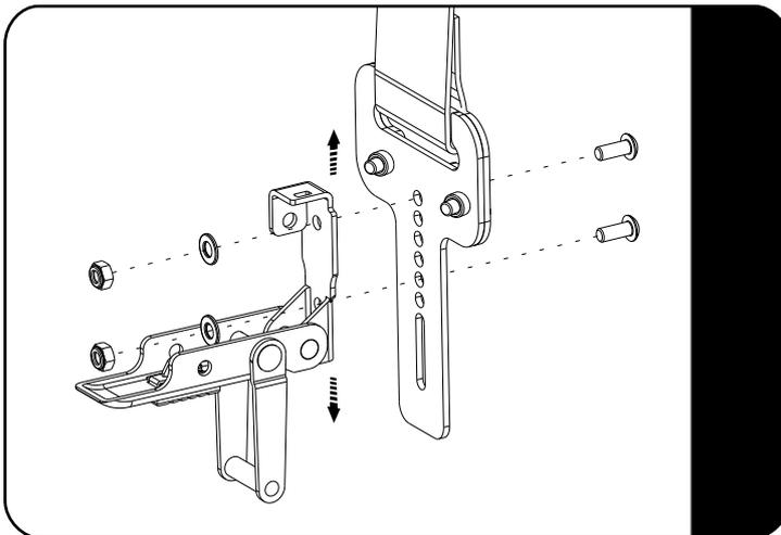
Using a 3mm allen key and a 7mm spanner, loosen the two bolts holding the latch to the latch plate.
