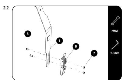
Loosely fit the Latch (Item 6) to the Top Strap (Item 1) using M4 x 8 Button heads, & M4 Nyloc Nuts (Items 5 & 7) as shown.
