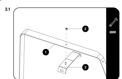
Secure the Cross Strap (Item 3) to the Top Strap (Item 1) using a M5 Nyloc Nut (Items 2) as shown.
