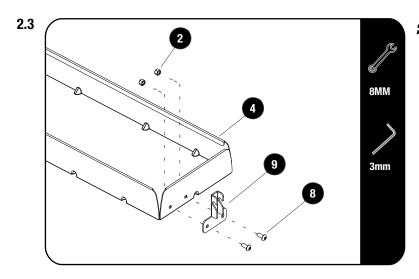
Secure the Latch Keeper (Item 9) to the Jerry Can Holder Base (Item 4) using two M5 x 12 Button Heads and Two M5 Nyloc Nuts (Items 8 & 2) as shown.
