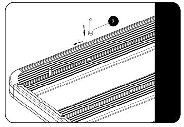
Slide two M8 x 35 Hex Bolts (Item 9 from) into the Slats machined slots on the underside of the rack.
