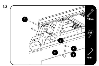
Loosely fit the Mounting Feet (Item 2) using M8 Flat Washers, M8 Nyloc Nuts and M6 x 45 Button Head Bolts (Items 4, 5 & 7) as shown.
