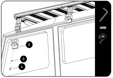
Place the assembled Tray with Legs onto the vehicle's gutters.
