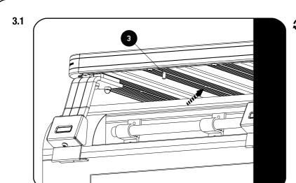
Slide M8 x 20 Hex Bolts (Item 3) into the machined slots on the 2nd, 6th & 9th slats from the rear.
