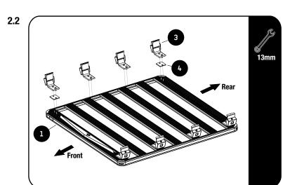
Loosely assemble the Legs & Spacers (Items 1, 3 & 4) as shown, slats indicated in 2.2 using M8 Flat Washers and M8 Nyloc Nuts included in the Leg sets.
