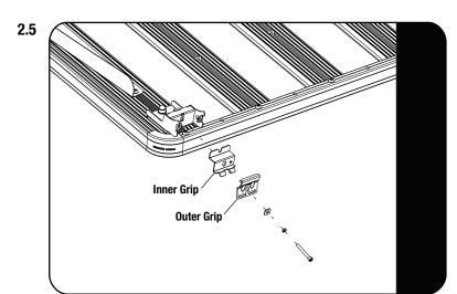
Loosley fit one Inner Grip and one Outer Grip to each Grab On Foot using a M5 Cap Screw, M5 Spring Washer and M5 Cap Screw Washer removed.
