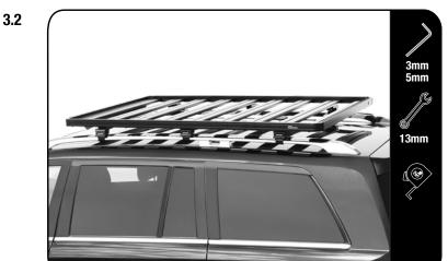
Place your Tray on the vehicle positioning all the feet so that they rest on top of the roof rails.
