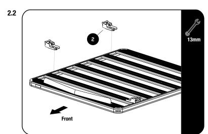
Loosely assemble the four Grab On Feet (Item 2) onto the slats indicated in 2.1 as shown using M8 Flat Washers and M8 Nyloc Nuts.
