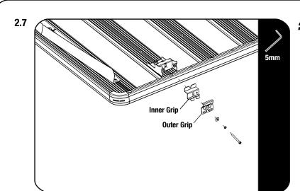
Loosley fit one Inner Grip and one Outer Grip to each Grab On Foot using a M6 Cap Screw, M6 Spring Washer and M6 x 20 x 2 Flat Washer.
