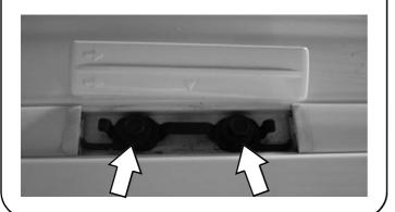
(**C**) Place a Spacer (Items 6) into each of the Mounting Point Recess, lining up the holes in the Spacers with the bolt holes in the roof. Ensure that the wide section of the Spacers (as indicated in the image) go towards the outside of the vehicle.
