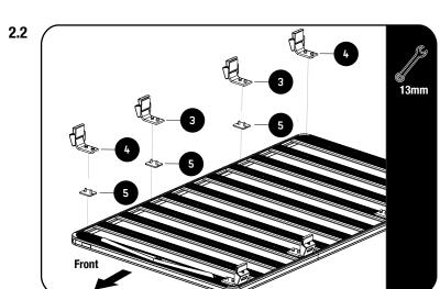
Loosely assemble the Legs & Spacers (Item 3, 4 & 5) as shown, slats indicated in 2.1 using M8 Flat Washers and M8 Nyloc Nuts included in the Leg sets.
