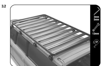
Place your Tray on the vehicle positioning all the feet so that they rest on the gutters.
