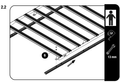
Ask a friend to help you place the rack onto the tracks of your canopy or trailer. Place the rack in a suitable positon and center it front to back and left to right before fully tightening all the M8 Nylock Nuts (Item6).
