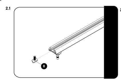
Slide 6 of the T-Bolt M8 x 20 / 18mm Wide (Item 8) into each side of the tracks on your canopy or trailer.
