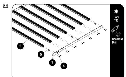
Slide the 4 M8 x 16 Hex Head Screws (Item 5) into the front, middle and rear Slim Sport Slat (Item 2). Attach the Footrail (Item 1) using the M6 x 25 Thread Forming Screws (Item 4).
