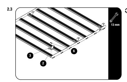
Flip the rack over and loosely assemble the Canopy Feet (Item 3) to the Slim Sport Slats (Item 2) using the M8 Nuloc Nuts (Item 6)
