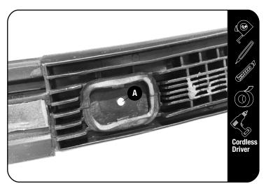
Peel back the weather strip enough so that you can remove the weather strip retaining bolt, Remove the Stud insert from the plastic trim and place the Bottom Spacer (Item 6) into the opening and mark the center of the hole (A).
