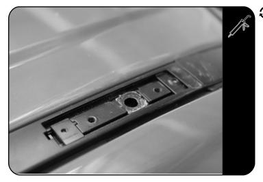
Place a bead of Sealant on the Ditch Trim before placing it back into the vehicles ditch.
