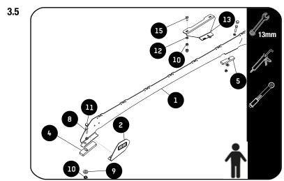
Apply a bead of sealant on the threads of the M8 x 40 Hex Bolts and secure the Foot Rail (Item 1) together with the Support Bracket (Item 13) and the Front and Rear Spacers (Item 4 & 5) to the Roof using M8 x 45 Hex Head Bolts, M8 x 19 x 2 Flat Washers and M8 Nyloc Nuts (Items 8,9 & 10).
