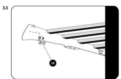
Remove the backing from the double sided tape on the bottom of the Support Plate (Item 4) before appliying the Spacer (Item 18) to the Support Plate.
