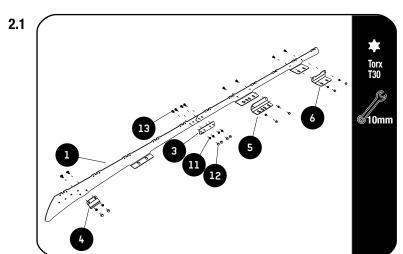
Secure the Joiner Plate (Item 3) to the Foot Rails (Items 1 & 2) as shown using M6 x 16 Flange Button Head Bolts and M6 Nyloc Nuts (Items 11 & 13).
