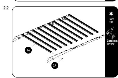
Fit 10 Slimsport Slats (Item 16) to assembly 2.1 using M6 x 25 Thread Forming Screws (Item 14).
