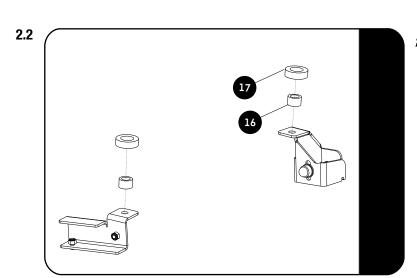
Once all the mounting Brackets are in place and fully tightened drill the holes from the bottom of the brackets using a 6mm drill bit.
