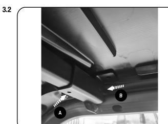
Place the Front Mounting Bracket (Item 6) onto the front Cross member and secure the Front mounting Bracket To the OEM hole (A) Using M6 x 12 Button Head Bolt and M6 Nyloc Nut (Item 14 & 15). Fully Tighten.
