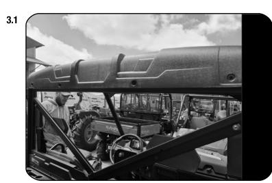
Start by removing the 4 bolts holding the roof in place to gain access behind the roof and keep aside to refit.
