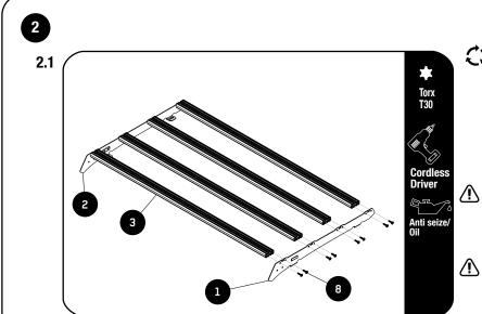
Fit 4 Slimsport Slats (Item 3) to the Foot Rails (Item 1 & 2) using 16 x M6 x 25 Thread Forming Screws (Item 8) as shown.
