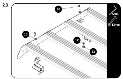
Secure the Tray to the Roof using M8 x 30 Button Head Screw, M8 x 19 x 2 Flat Washers and M8 Nyloc Nut. (Items 10, 12,18).
