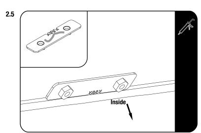
Apply a bead of sealant on the six Nut Plates (Items 6 & 7), and secure the Slimsport Roof Rack to the Nut assemblys as shown in Step 2.6. This will allow easy removal of the rack in the future.
