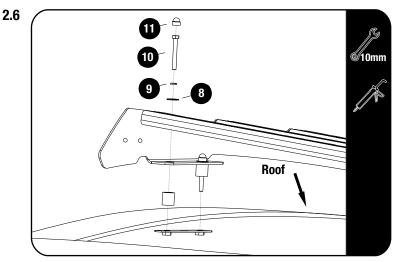
Apply Sealant over the 12 holes on the outside of the roof.
