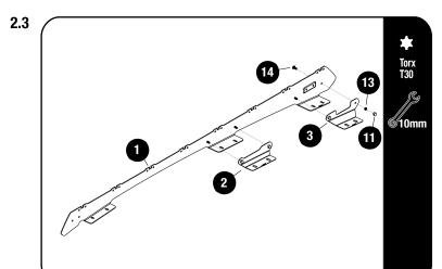
Secure the stiffener plates (Items 2 & 3) to the Foot Rails (Item 1), using M6 x 16 Flange Button Heads & M6 Nyloc Nuts (Items 13 & 14). Fully tighten.
