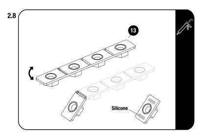
Twist the nut plates (Item 13) free from each other and apply silicone before the fitment in step 2.7.
