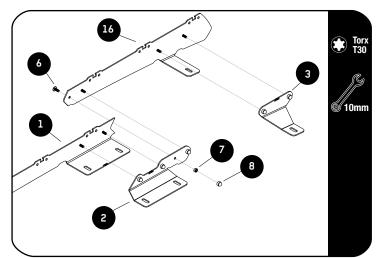
Join the Front LH and Rear LH Foot Rails (Item 1 & 16) with the Middle Stiffener Plate provided (Item 2) using M6 x 16 Button Head Flange Bolts and M6 Nyloc Nuts (Items 6 & 7).
