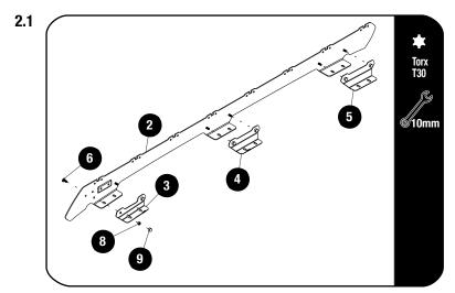
Secure the stiffener plates (Items 3, 4 & 5) to the Foot Rails (Item 2), using M6 x 16 Flange Button Head Screws & M6 Nyloc Nuts (Items 6 & 8). Fully tighten.
