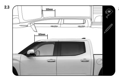
Measure 325mm backward from the top edge of the winscreen and make a mark, do this on both the LH / RH ditch.
