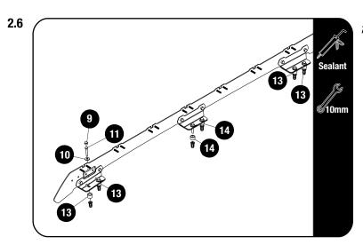
Place the tube spacers (Item 13 & 14) into the mastic of all holes drilled, 2 x 15mm spacers in the front holes 2 x 12mm spacers in the middle holes and 2 x 15mm spacers in the rear holes. Fill the tube spacers with silicone sealant.
