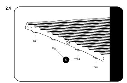
Place a bead of silicone around the exisiting mounting points from 2.2.
