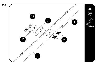
Assemble the Front and Rear Foot Rail (Items 1 & 5) with the Joiner Plate (Item 7) using M6 x 16 Flange Button Head Bolts and M6 Nyloc Nuts (Items 9 & 10) as shown.
