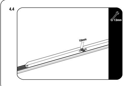
Center the Wind Deflector on the rack and move the bolt assemblies from fig 4.1 into the slots as shown in fig 4.4.
