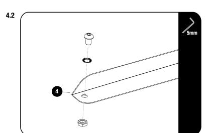
Loosely assemble the M8 x 12 Button Head Bolt, M8 Schnorr Washers and M8 Thin Nut both LH & RH Wind Deflectors (Item 4) as shown.
