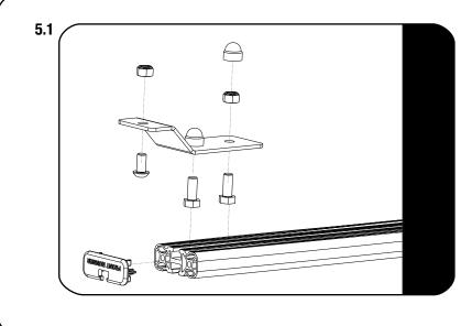
Loosely assemble the Slat Z Brackets (Item 3) to the Narrow Slats using M8 x 20 Hex Bolts and M8 Nyloc Nuts.
