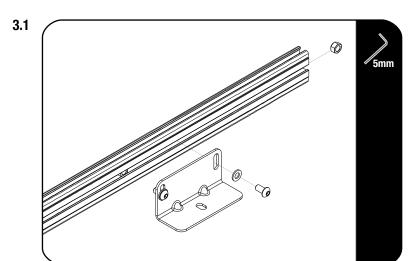
Loosely assemble the Ford Transit Feet (Item 6) using M8 x 16 Button Head Bolts, M8 Flat Washers and M8 Nyloc Nuts and slide them into the side profiles. They must still be able to slide freely.
