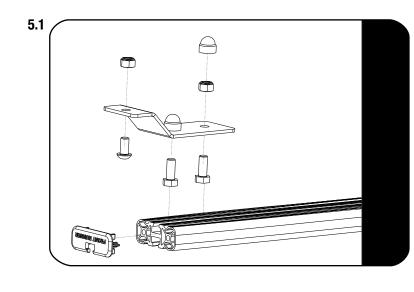
Loosely assemble the Slat Z Brackets (Item 2) to the Narrow Slats using M8 x 20 Hex Bolts and M8 Nyloc Nuts.
