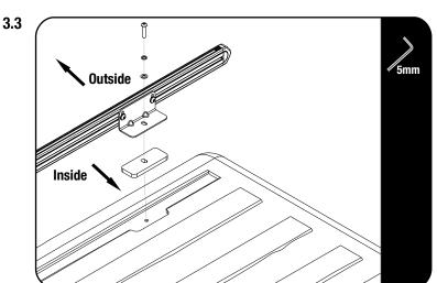
Apply Sealant around all mounting holes in the roof.
