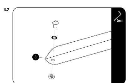
Loosely assemble the M8 x 12 Button Head Bolt, M8 Schnorr Washers and M8 Thin Nut both LH & RH Wind Deflectors (Item 3) as shown.
