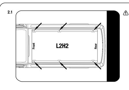
Locate the factory mounting points on the vehicle's roof.
