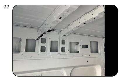
In 3.3 you will use these access points to secure the feet to the roof.
