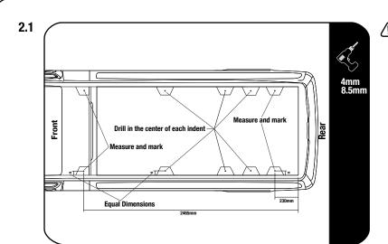
Note the indents on the 6 center positions on the roof. Drill a 4mm pilot hole in the center of each indent. Open the pilot holes to 8.5mm
