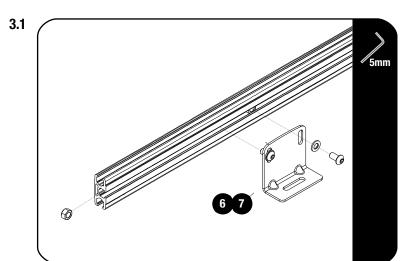
Loosely assemble the Feet (Item 7) using M8 x 16 Button Head Bolts, M8 Flat Washers and M8 Nyloc Nuts and slide them into the side profiles. They must still slide freely.
