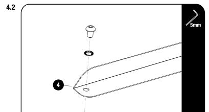
Loosely assemble the M8 x 12 Button Head Bolt, M8 Schnorr Washers and M8 Thin Nut both LH & RH Wind Deflectors (Item 4) as shown.
