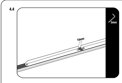
Center the Wind Deflector on the rack and move the bolt assemblies from fig 4.1 into the slots as shown in fig 4.4.
